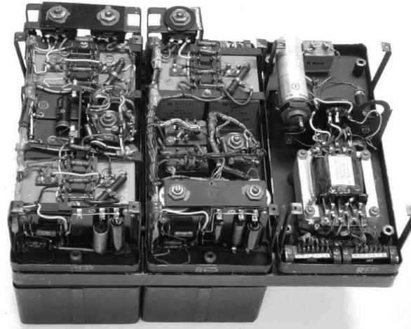
Mischgeraet : the world's first on-board computer, guidance section of V2 rocket.
