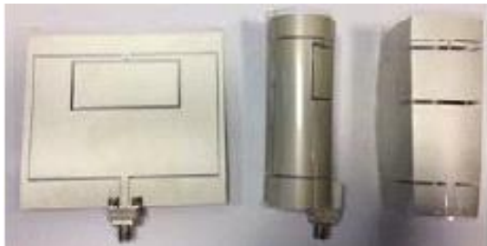
Coplanar antennas, without and with folding
