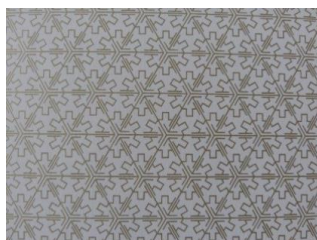
Tri-band Wifi rejected 0.97GHz, 2.25GHz and 3.14 GHz
