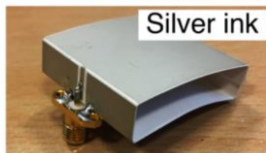
Wi-Fi antennas at 2.45 GHz with air gap
