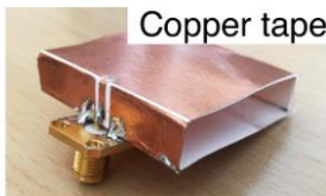
Wi-Fi antennas at 2.45 GHz with air gap
