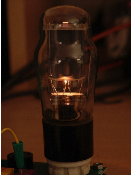
5Y3GB (1937) – full-wave rectifier 5V, 1.6A → 8W for the filament!
